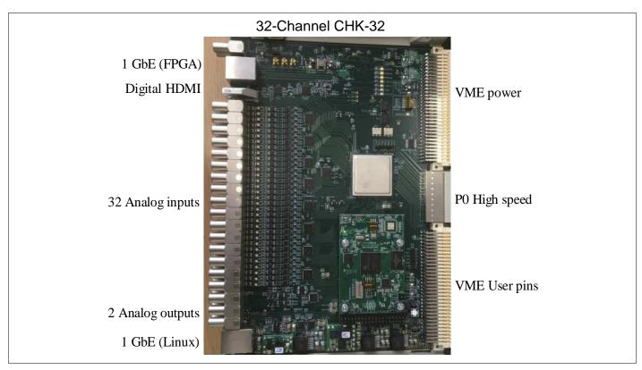
CHK-32 is a compact, high performance data acquisiton system. It uses a Linux Single Board Computer for control. It provides 32 digitizer channels and logic I/O for connecting to external devices. The analog inputs can be used with HPGe, silicon photomultiplers, PIN diodes, and other similar detectors.
